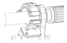
3. Link the cable from controller panel (B) and the cable from E-Bus (A) onto the display.
