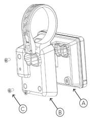
Open the clamps of display and place the display on to the handlebar in the correct position. Now with M3\*14 screws (A) tighten the display into position. Torque requirement: 0.3N.m.
